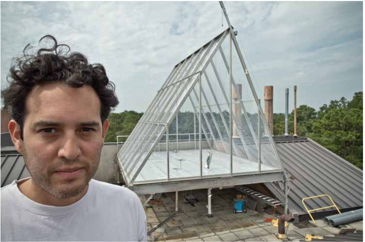
This smog chamber helps William Vizuite and his colleagues at the UNC Gillings School of Global Public Health create nearly any kind of atmospheric concoction they can think up. They can pipe it into a lab and test the effects of pollution on human cells. Now they want to take their show on the road. Photo by Mark Derewicz.
